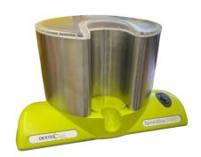
Dexter LifeSep® magnetic bead separators and products are designed to work with most commercially available superparamagnetic beads, roughly 0.8 micron and above. For beads in the nanometer range, we can provide extremely high-gradient, custom separation solutions achieving efficient collection that might otherwise only be possible with matrix-based technology.
